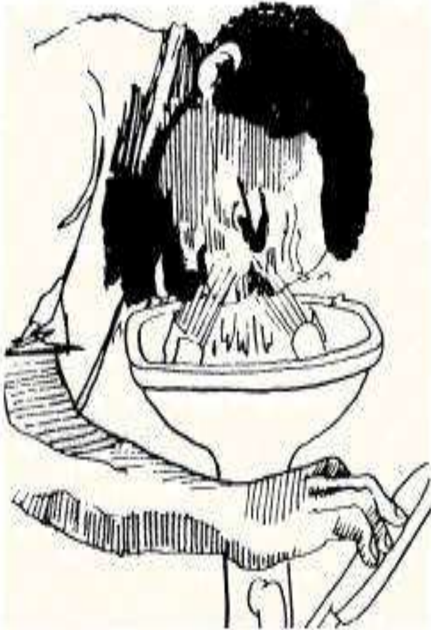
Figure 56. Emergency showers and eye-wash points should be provided in close proximity to workstations where hazardous chemicals are used
